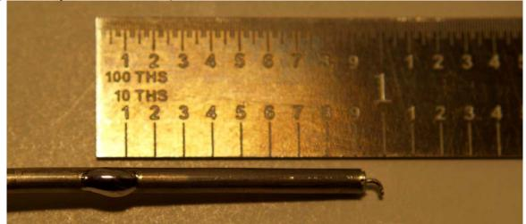
▷ Form the loop around a 0.25" diameter mandrel. I find the 0.25" diameter a convenient compromise between sensitivity, spatial resolution, and ease of probing. It provides a predictable response to ~1GHz.
