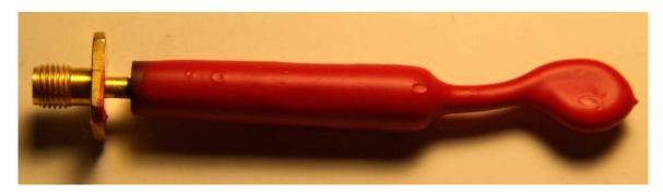
The probe is not perfect; it does not have a flat response with frequency, and it can also pick up E fields. It will certainly be far more sensitive at high frequencies, as it is a simple loop probe whose output voltage is given by Faraday's law. Faraday's law of induction (for a sine wave):
